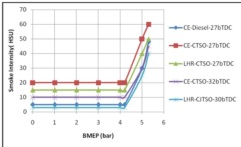
**Figure 8: Variation of Smoke Levels with BMEP in Both Versions of the Engine at Recommended and Optimized Injection Timings with CTSO Operation at an Injection Pressure of 190 Bar**
