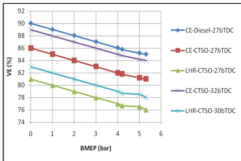
**Figure 7: Variation of Volumetric Efficiency (VE) with BMEP in Both Versions of the Engine at Recommended and Optimized Injection Timings with CTSO Operation at an Injection Pressure of 190 Bar**
