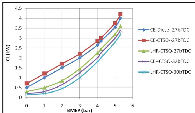
**Figure 6: Variation of Coolant Load (CL) with BMEP in Both Versions of the Engine at Recommended and Optimized Injection Timings with CTSO Operation at an Injection Pressure of 190 Bar**
