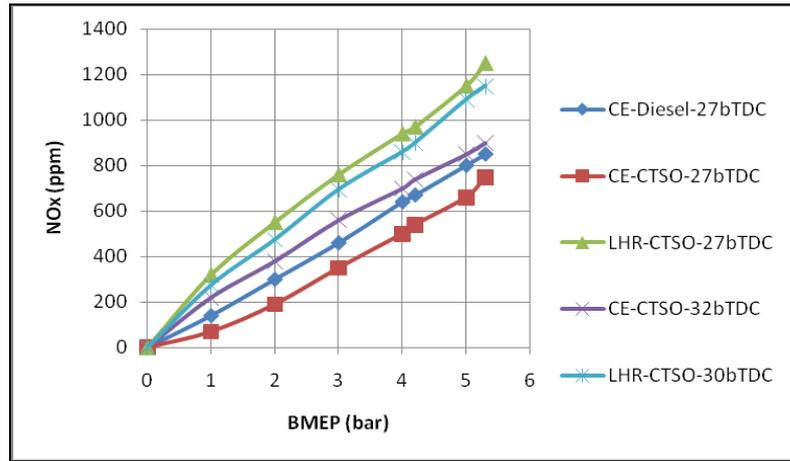
**Figure 9: Variation of NOx Levels with BMEP in Both Versions of the Engine at Recommended and Optimized Injection Timings with CTSO Operation at an Injection Pressure of 190 Bar**
