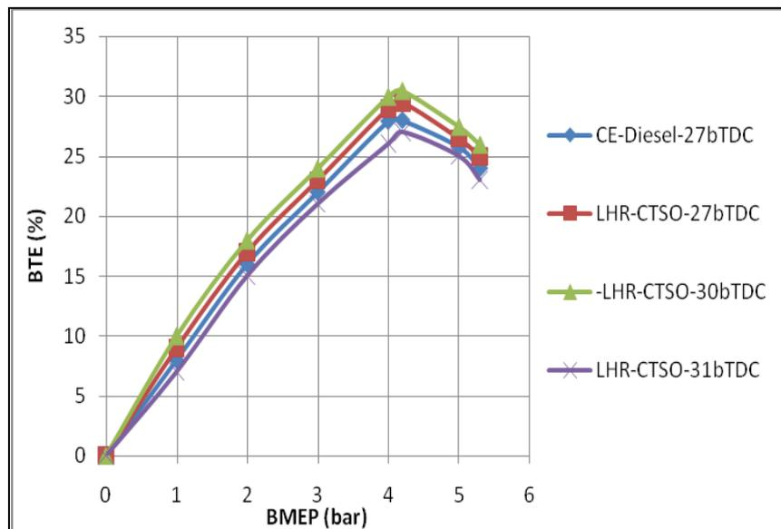
**Figure 3: Variation of Brake Thermal Efficiency (BTE) with Brake Mean Effective Pressure (BMEP) in LHR Engine with CTSO Operation at an Injection Pressure of 190 Bar**
