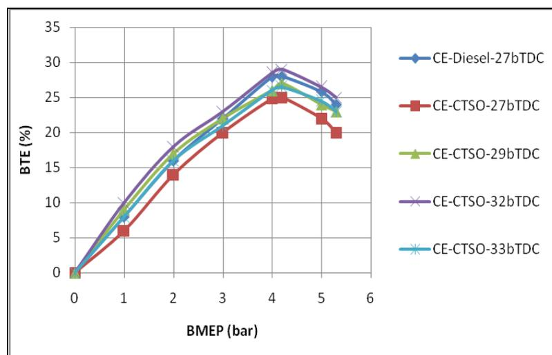
**Figure 2: Variation of Brake Thermal Efficiency (BTE) with Brake Mean Effective Pressure (BMEP) in CE with CTSO Operation at an Injection Pressure of 190 Bar**
