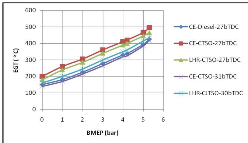
**Figure 5: Variation of Exhaust Gas Temperature (EGT) with BMEP in Both Versions of the Engine at Recommended and Optimized Injection Timings with CTSO Operation at an Injection Pressure of 190 Bar**
